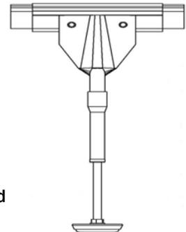
4. Center one clamp over the 2 angles, and extend the angles to the proper width so they rest on the cleats of the wood rails.
